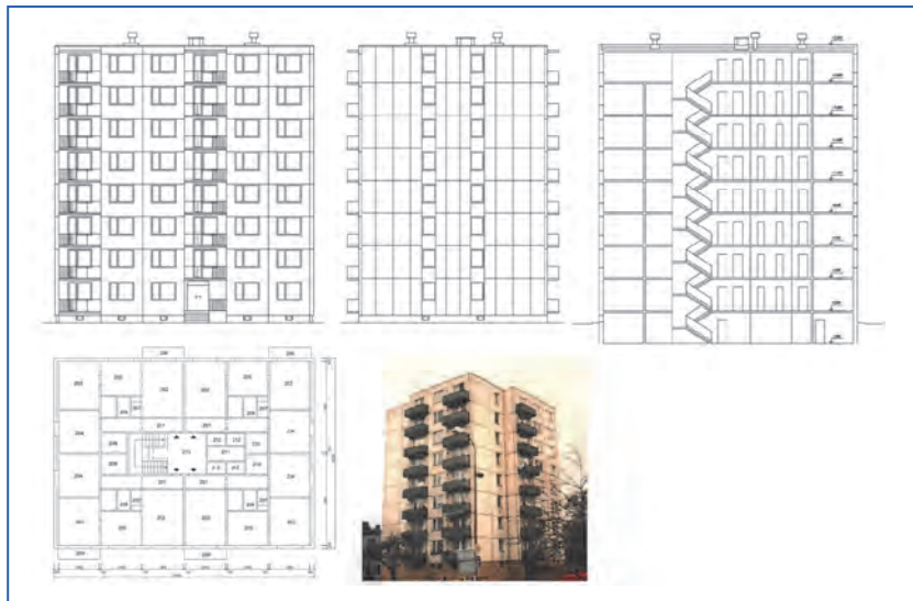
Figure 23.11. Multi-family house, tower type T06B-NR (porous concrete panel), [4].
