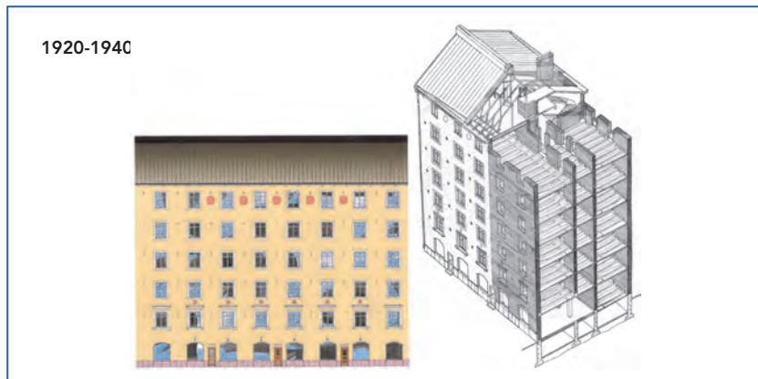
Figure 7.15. Example of a dwelling constructed in 1928. Left: façade 1:250, right: cross section. Typical structures: floor: inverted beam, walls between dwellings: double “Lugino mix” wall (an outdated mixture of slag, gypsum, sand and water) [5].
