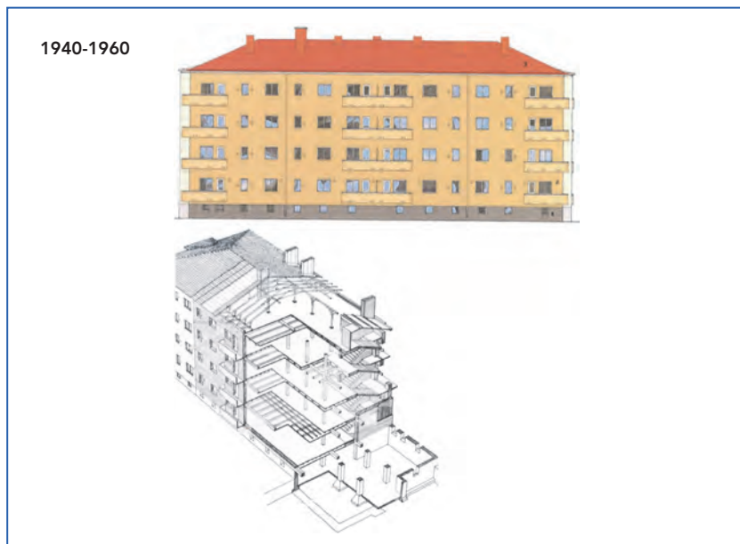
Figure 7.16. Example of a dwelling constructed in 1946. Top: façade 1:250, bottom: cross section. Typical structures: floor: inverted beam, walls between dwellings: “Riksi-board” wall (an outdated mixture of woodchips and gypsum) [5].
