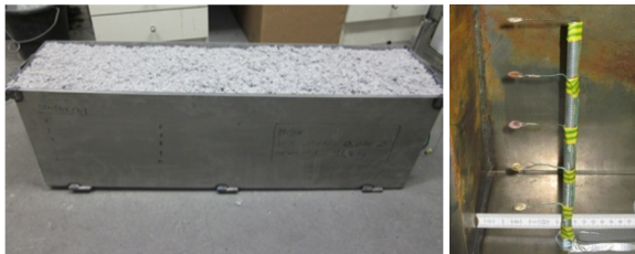
Figure 1. Cellulose insulation sample before testing and thermal elements in the sample box
