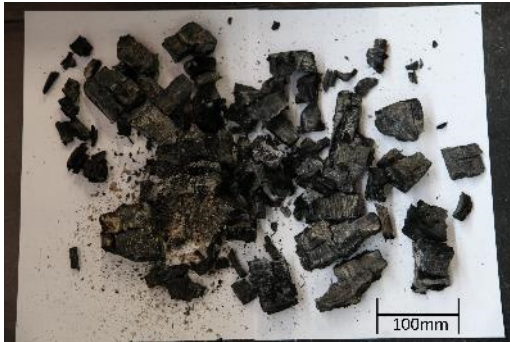
Figure 3. Delaminated pieces from H-TRIS test H3-100-1
