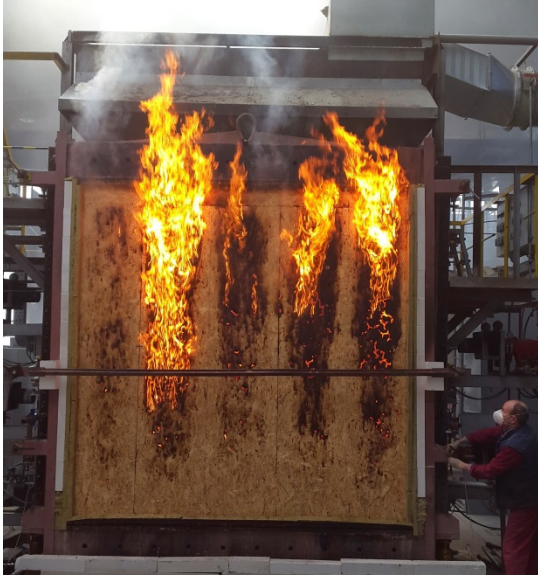
Figure 1. One layer cladding with empty cavity.
