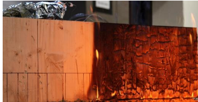
Figure 4. Extent of flaming prior to delamination in flame spread test, 235s into test
