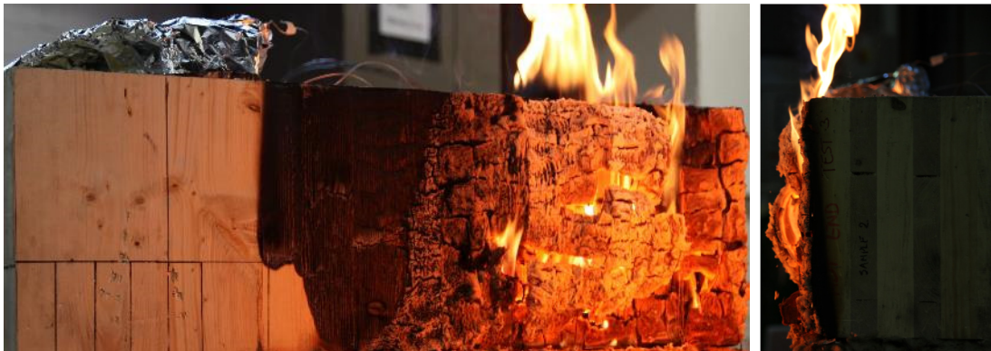
Figure 5. Flaming between lamellae in flame spread test, 2380s into test
