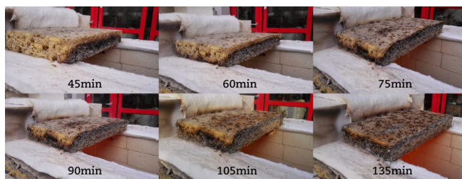
Figure 3. Fire performance of 50 mm prefabricated WLC noise protection chipboard.
