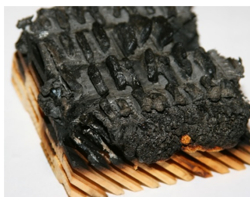
Figure 4. Intumescent fire retardant effect on cellular wood combustion "D+A5".
