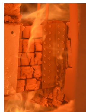
Figure 3. Loaded fire test with joist hanger.
