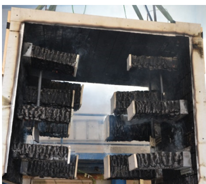
Figure 1. Unloaded test specimen after fire exposure.
