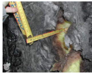
Figure 4. Glass wool after 54 min fire test, [4]
