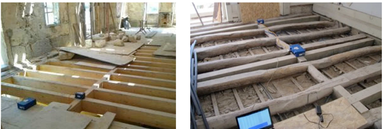
Figure 6: Dynamic identification of timber floors (without floorboards)
