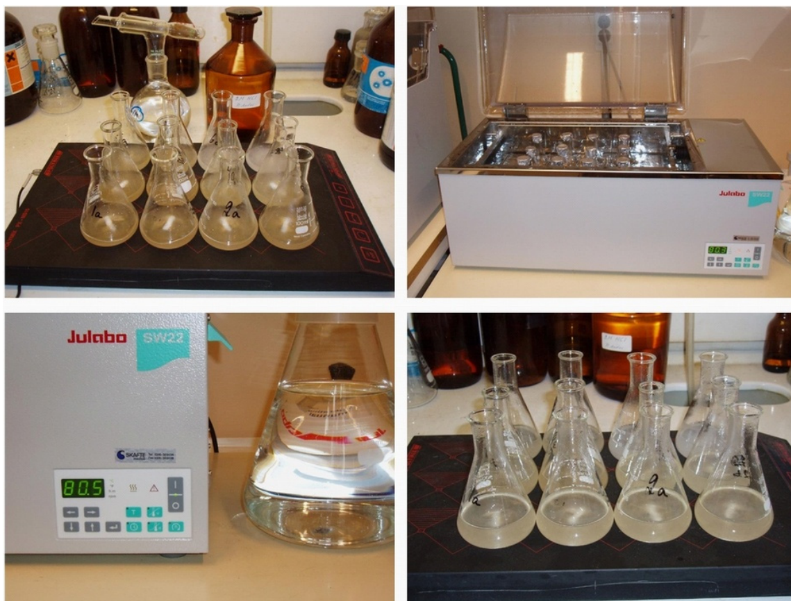
Figure 3. Procedure steps of the HCl-method for fiber cleavage: Swelling of fibers in 20 mL water with stirring (above left), shaking fiber in 1M HCl for 4 h at 80-81°C in the water bath - plastic lid closed during treatment (above right), close up of water bath (below left), and cooling down with stirring for 30 min (below right)
